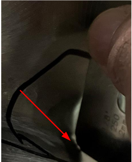
WM-36 W-13, Undersized weld ~ 1-1/2" long section
