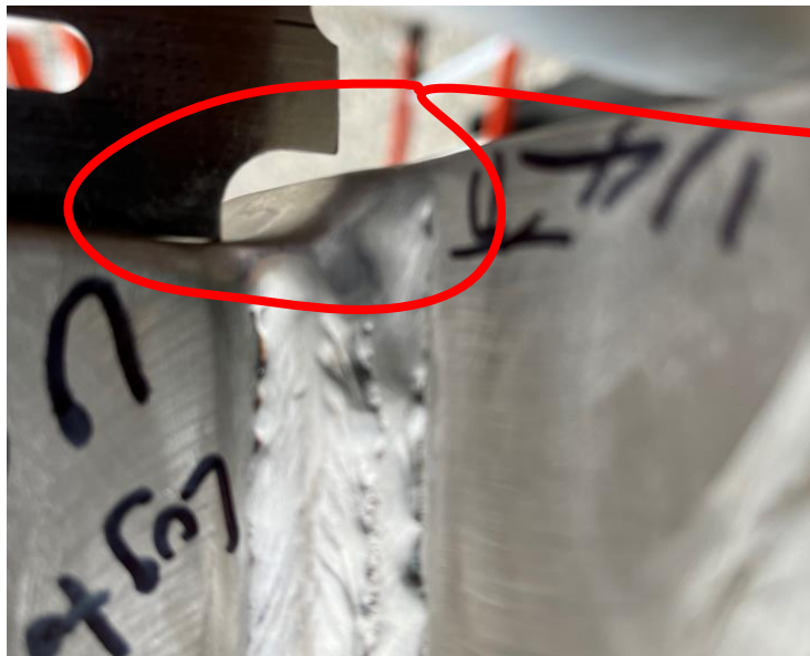
WM-25 W-6, 7 & 8 - 3/8" fillet weld not achievable. Configuration of lug to head only permits 1/4" fillet on Outside edge of lug to Top head Flange.
