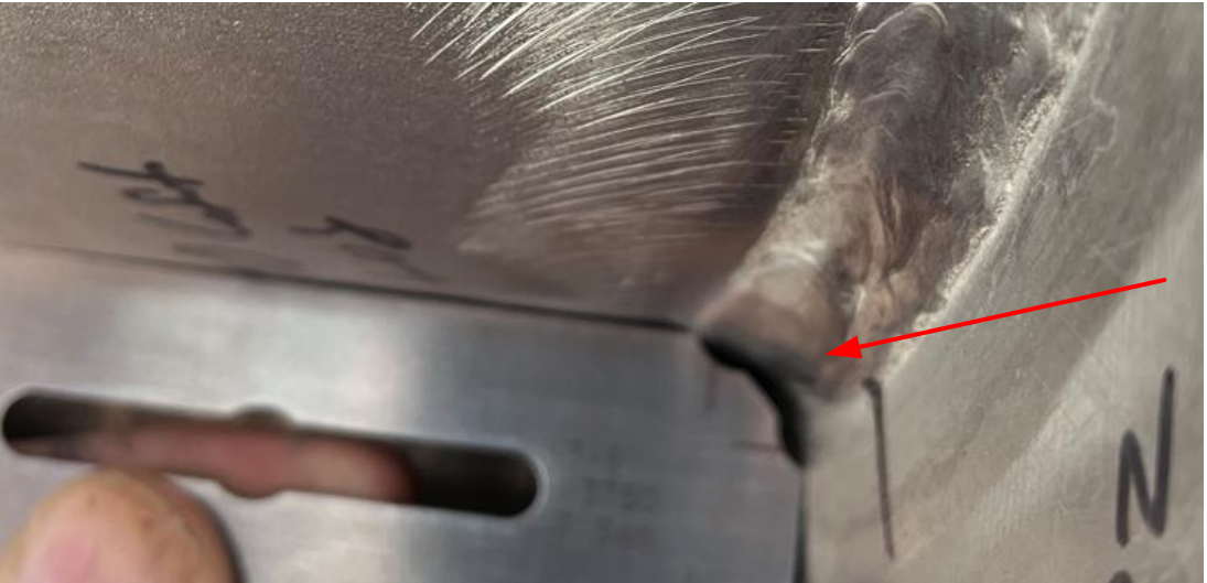
WM-32 W-2, Insufficient throat for ~ 1-1/2" segment at 8 O'clock
