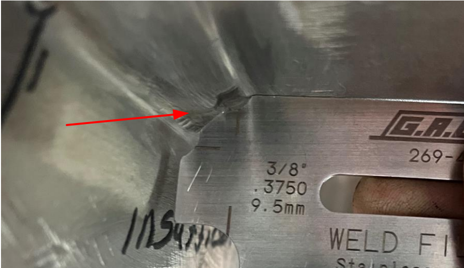
WM-32 W-1, Insufficient throat at 1-3 & 4-5 O'clock
