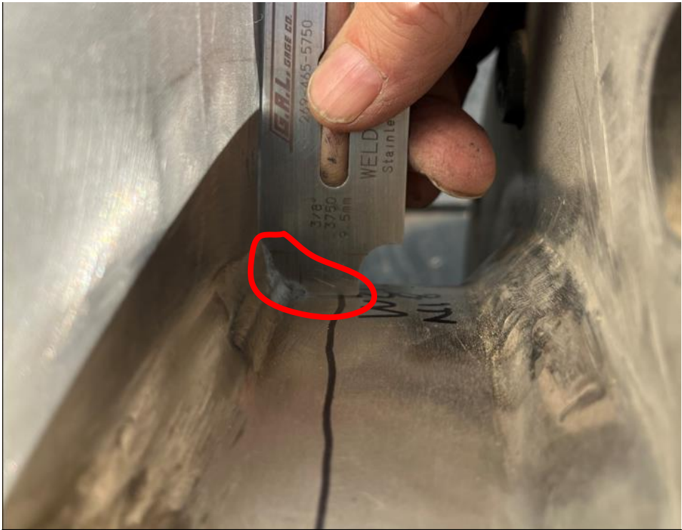
WM-26 W-21 Insufficient weld throat by ~ 1/16" between 7 to 1 O'clock
