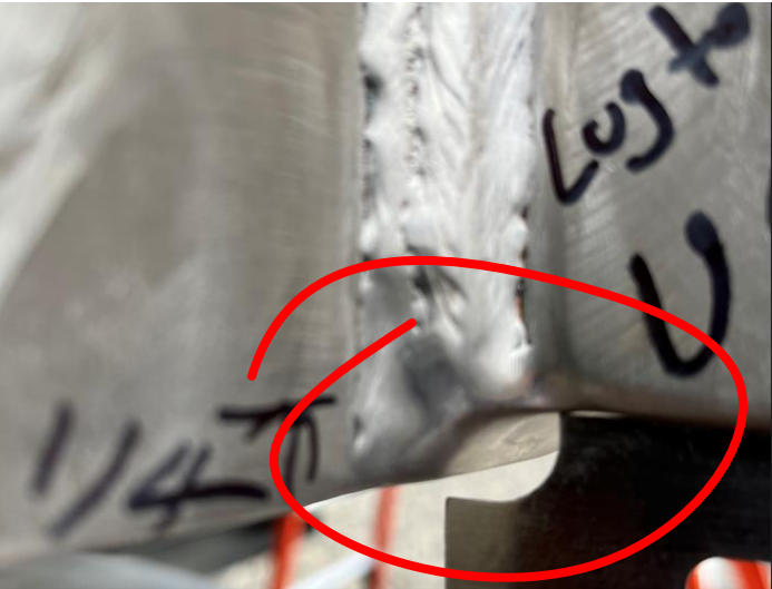
WM-34 W-6, 7 & 8 undersized at end, 3/8" is not achievable
