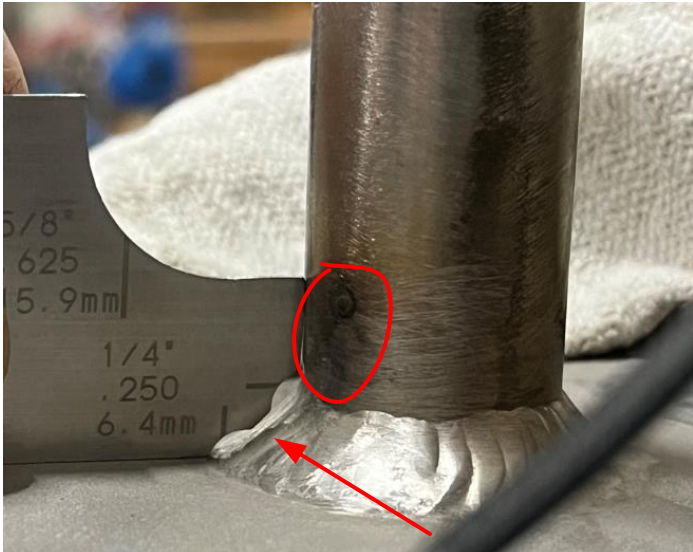
WM-36 W-18, Undersized weld Throat & arc strike
