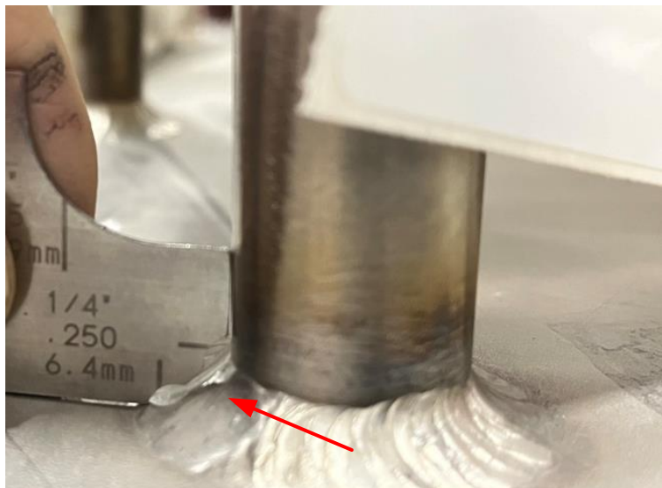
WM-36 W-19, Undersized weld throat
