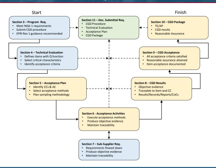
Specification T0019, revision 2, is organized around this CGD process map. Each step of the map provides reference to corresponding sections of the specification.
