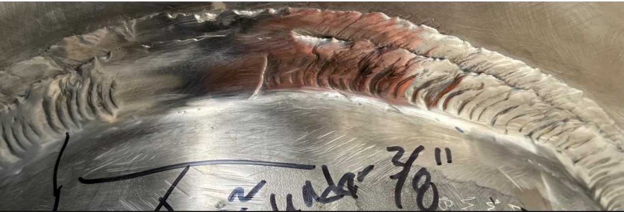
WM-31 W-5, Weld undersized @ 11:30- 2 and 4-5 O'clock
