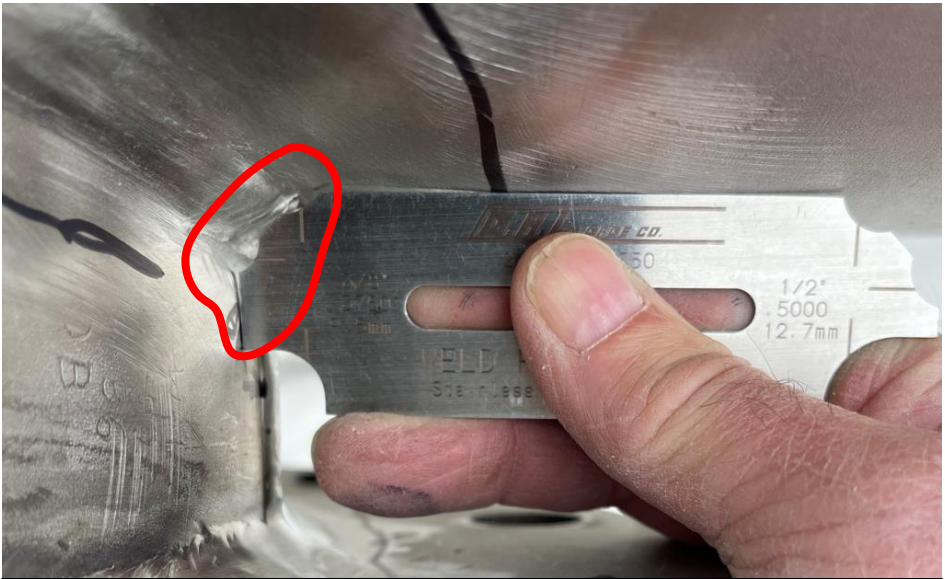
WM-26 W-23 Undersized weld by ~1/16", & Insufficient weld throat
