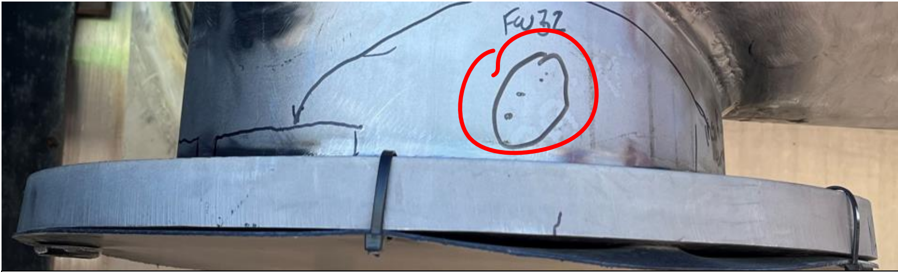
WM-26 W-32 Undersized weld, & Insufficient weld throat ~ 90% of over-all weld length
