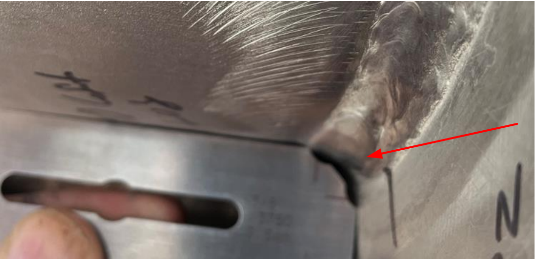
WM-32 W-2, Insufficient throat for ~ 1-1/2" segment at 8 O'clock
