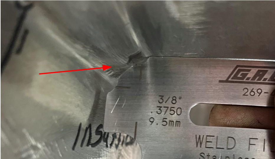
WM-32 W-1, Insufficient throat at 1-3 & 4-5 O'clock
