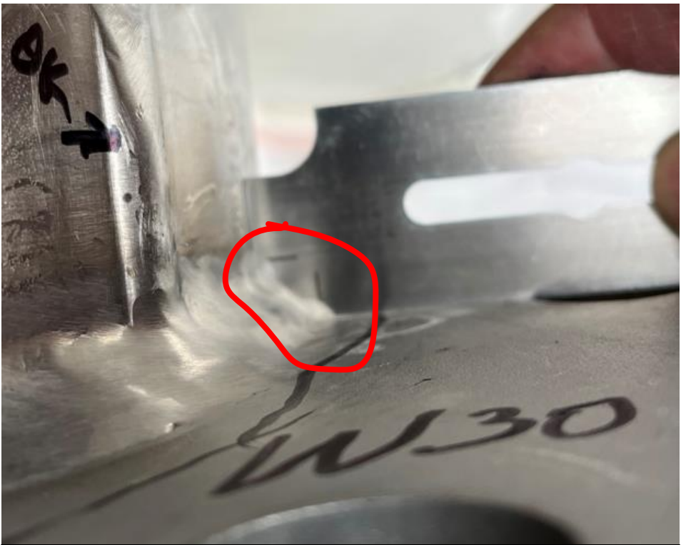
WM-26 W-30 Undersized weld by ~ 1/16", & Insufficient weld throat
