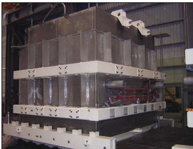
When operational, the WTP will contain two 90-ton high-level waste melters. The melters, which heat the waste mixture to high temperatures before it is poured into stainless steel canisters for permanent storage, are central to the vitrification process.
